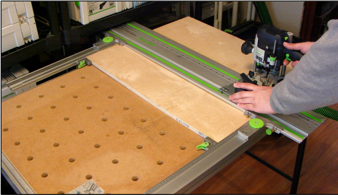
Here I'm exploring the idea of using the guides with the LR 32 hole drilling system.
