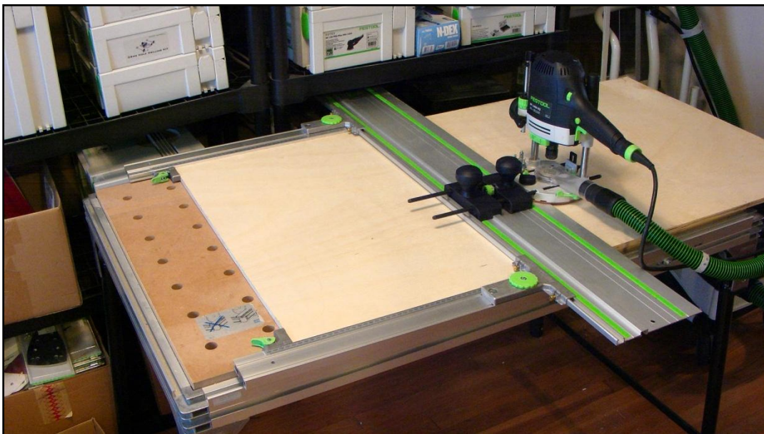
The guides can also be used to set the rail to precise measurements for routing applications.
