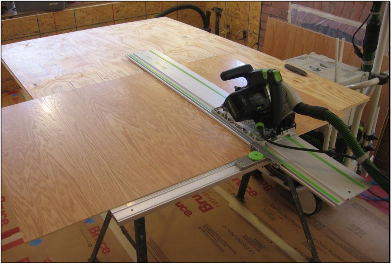
The FS-PA can be used to make 90° cuts, here I'm using just one of the guides.
